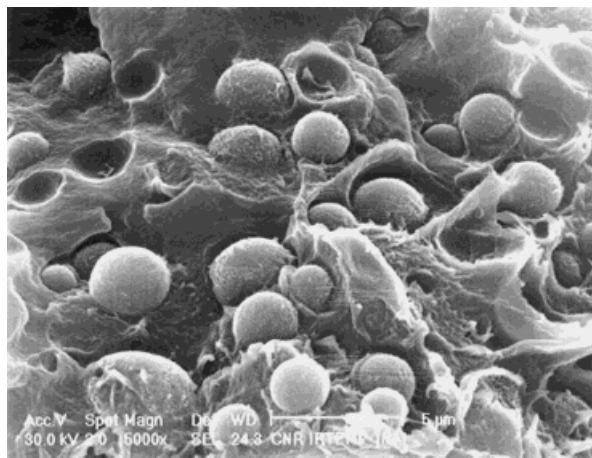
Figure 9 SEM micrographs of cryogenical fracture surfaces of iPP/aPS/uPP- g -PS ternary blends containing 5% (wt/wt) of uPP- g -PS copolymer (5,000 \times ).
